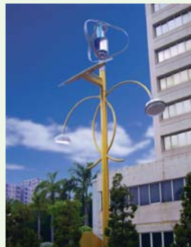
Step-by-step introduction of solar and wind power generators to reduce the level of greenhouse gas emissions.
